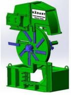
"Replace and Run" components supplied from Canada. Bearings and Cylinders supplied from Canada (Blue items) Steel structure and Chipper Disc sourced in China (Green items) Cost savings of 30% compared to North American manufacturing
